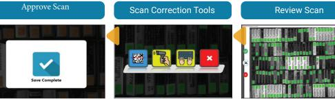
Upon operator approval, the data set and reference image are automatically stored to the **Path**Tracker database and posted to the LIS tracking system.
